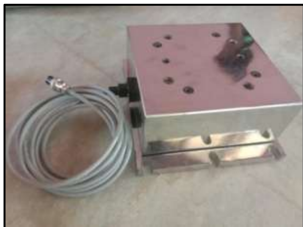
Fig. (4) V-TECH Grinding Tool Dynamometer- Model 220B sensor.
